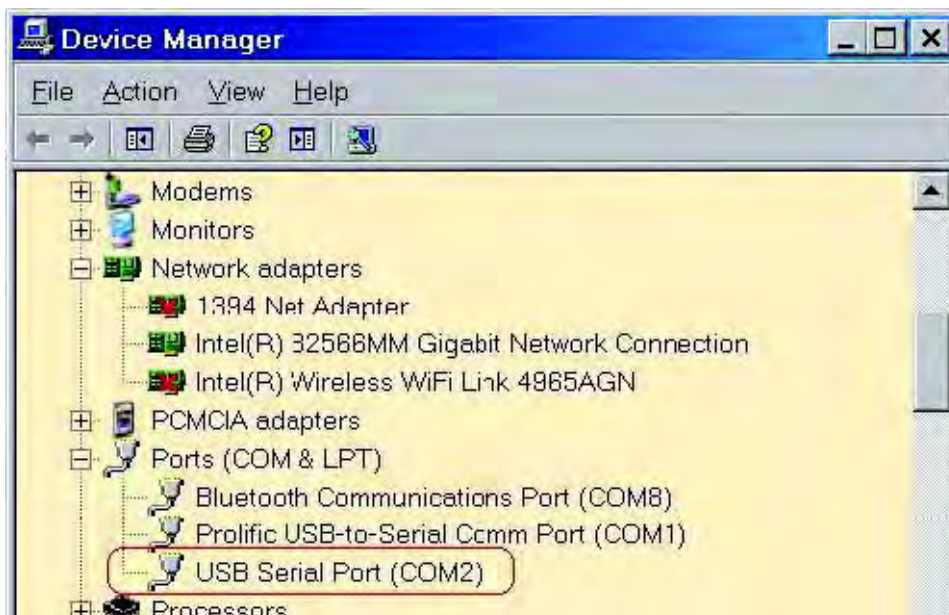
Figure 2. A Successful USB-to-UART Driver Installation
