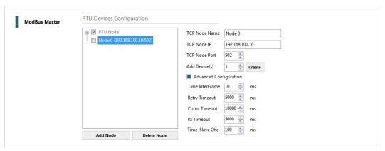
Fig. 27 Modbus TCP node configuration
