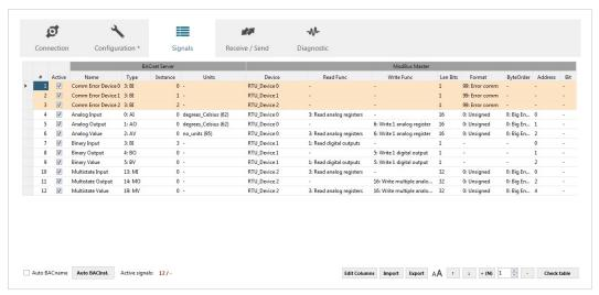
Fig. 30 Modbus signals
