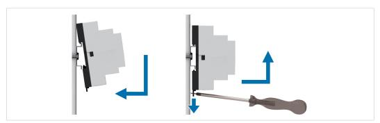
Fig. 3 DIN rail mounting option
