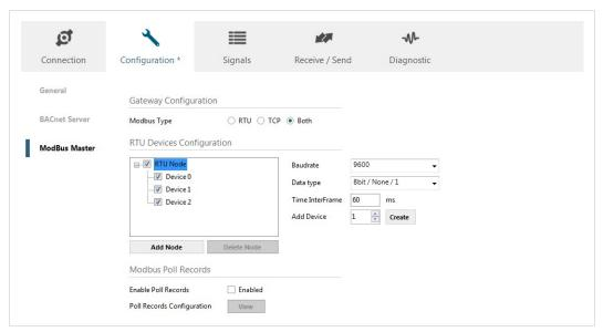
Fig. 24 Modbus master configuration
