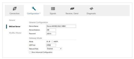
Fig. 11 BACnet configuration
