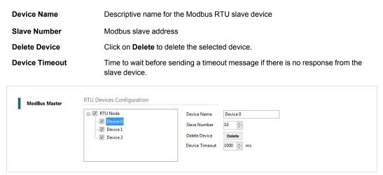
Fig. 26 Modbus RTU node configuration
