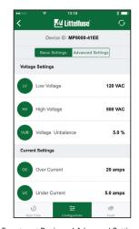
Easy to set Basic and Advanced Settings. Stand next to the motor and enter the motor specs right into the app to save set-up time.
