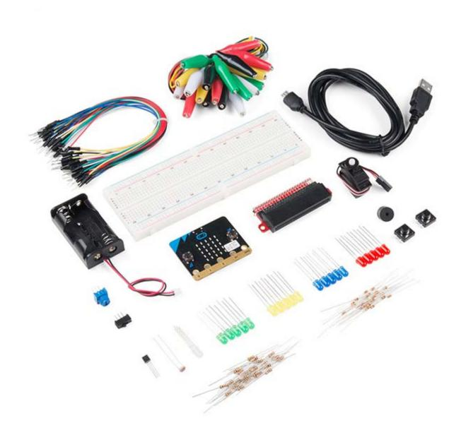
**Description:** The SparkFun Inventor's Kit (SIK) for micro:bit is a great way to get creative, connected and coding with the micro:bit. The SIK for micro:bit provides not only the micro:bit board but everything you need to hook up and experiment with multiple electronic circuits! With the SIK for micro:bit you will be able to complete circuits that will teach you how to read sensors, move motors, build Bluetooth devices and more.
