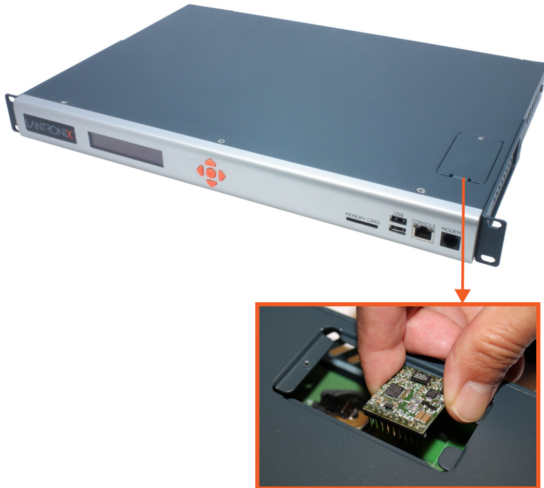
Figure 2-14 Internal Modem Location
