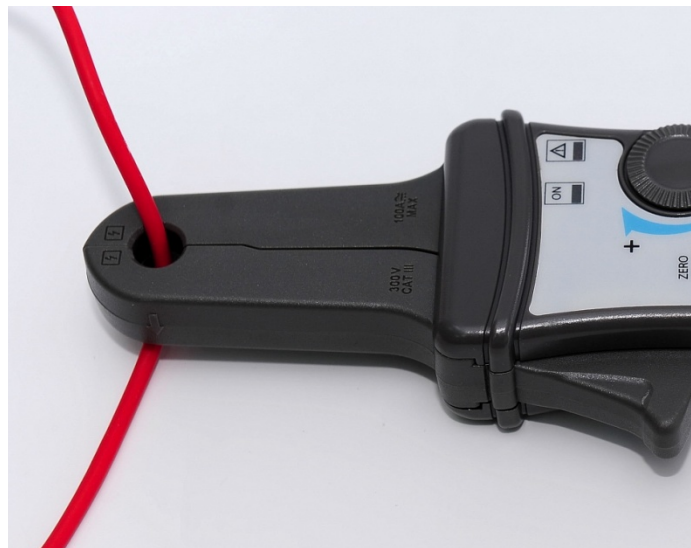
Figure 5: Connecting the CP62 current probe.
